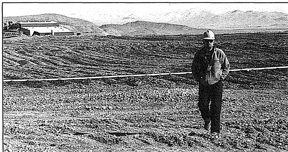
Tom Crafford, Exploration Manager of North Pacific Mining Corporation, stands before a drip tube application of dilute cyanide solution at a heap leach operation in Nevada.
