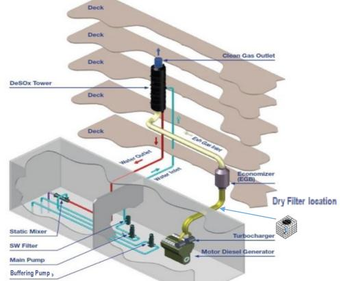
Between DeSOx tower and filters, over 98% of particulate matter can be removed.
