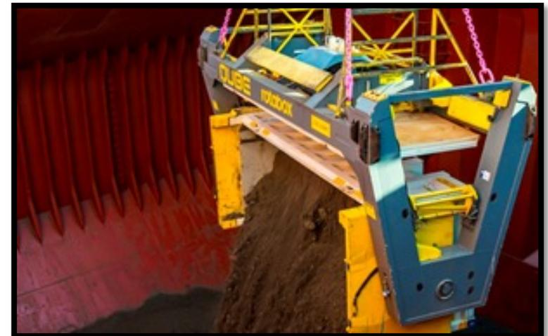
*Revolver tipping container in ship's hold*
