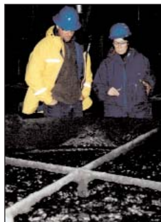
Greens Creek employs a flotation system to extract the silver, lead and zinc.
