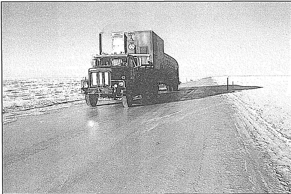
RDC recently urged the Alaska State Pipeline Coordinator's Office to approve right-of-way leases for pipelines associated with the development of ARCO's new Alpine oil field. RDC noted the pipelines would have only a very small footprint and would be built by crews using ice roads. Pictured above is an ice road built last winter for the Alpine project.
